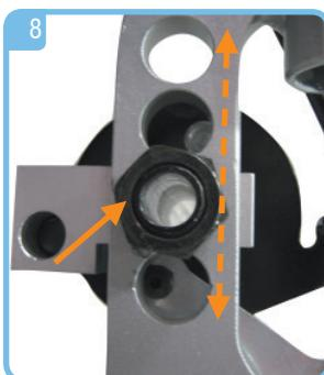
**⚠ Make sure the nut is securely tightened!**
